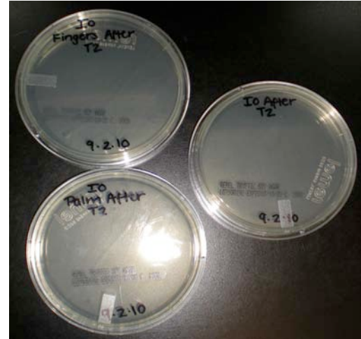
Figure 4. Close up of INSTANT-OFF replicates after the hand washing simulation. From left to right: Fingertips (top) and Palm, Instant-Off actuator rod. No E. coli K-12 colony forming units were recovered.
